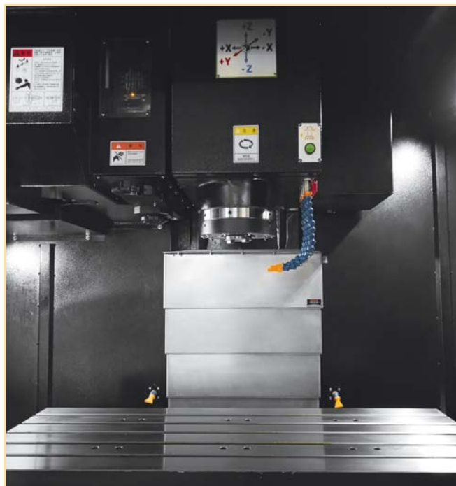
Keyarrow telescopic covers in all axes
