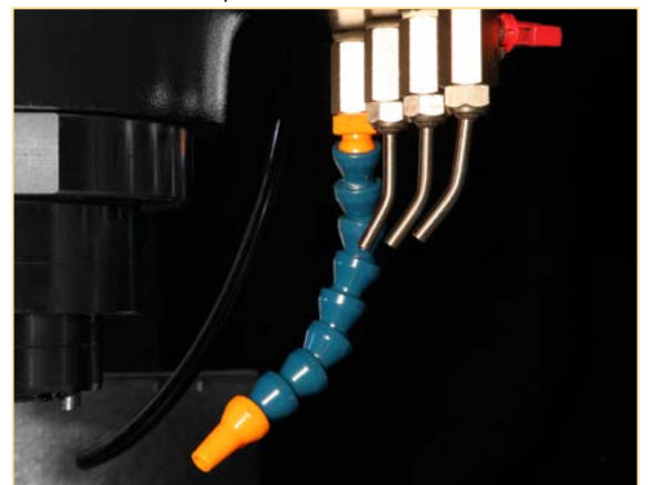
External tool cooling
